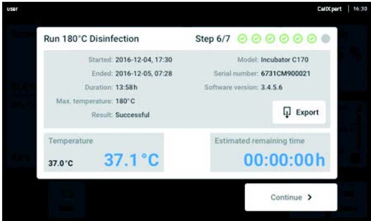
Fig. 10-11: Display of the result of the HTD after achieving the target temperature
