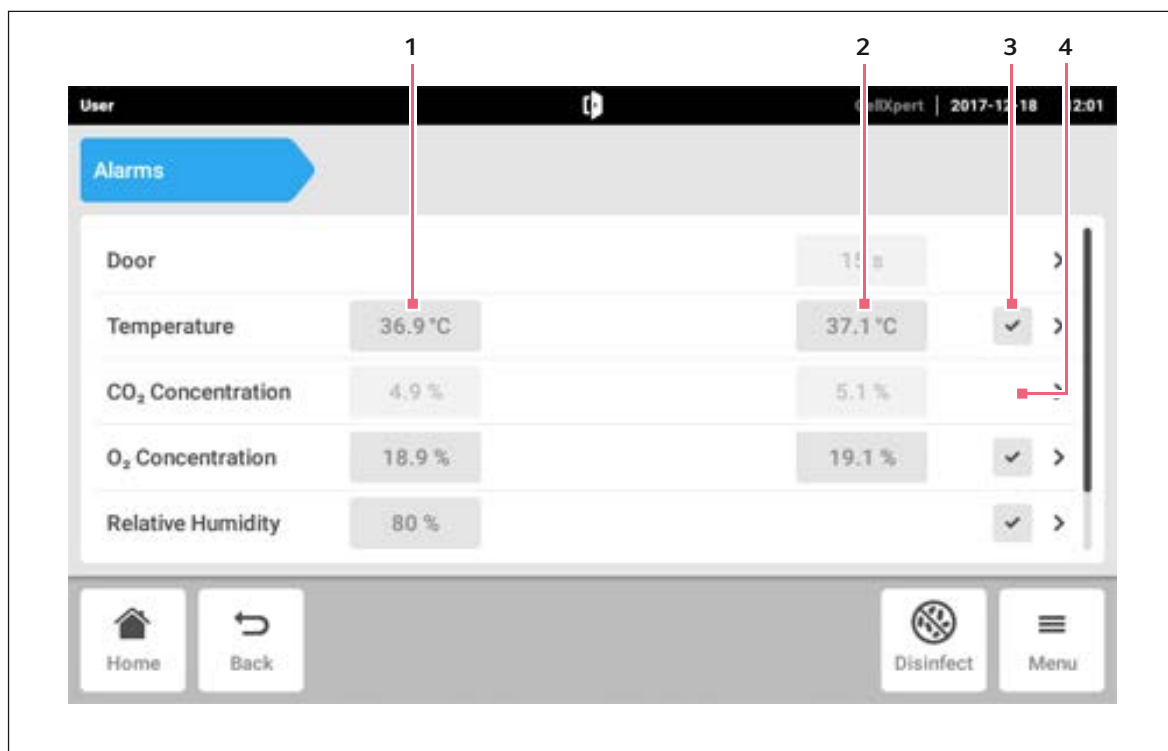
Fig. 8-6: Overview with device alarms, warning limits and alarm limits
